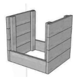
Fasten the remaining 6 boards to form the end walls..
